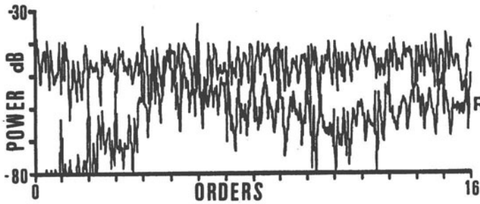
Figure 4 Order spectra for the bearing inner race defect (R = reference bearing)
