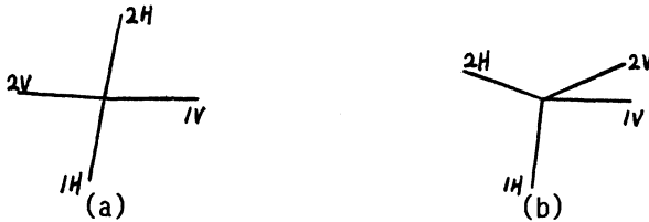
Fig.8. The phase differences among different measuring points. (a) A \text{CO}_2 -compressor, (b) An air-compressor.
